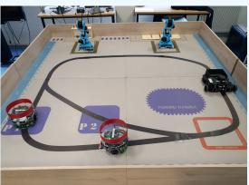
The first Niryo robot carefully grasps a battery from a "shelf" and puts it in the rectangular box of the ISEN robot, which goes on its way to the second manipulator to receive the screws. While the first mobile robot does its work, the other one waits patiently to subsequently take action.
