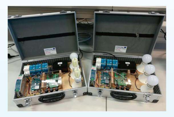
We examined the feasibility of PLC, focusing on outages and electromagnetic interference (EMI). Interference arises because each electronic product emits electromagnetic fields, desired or otherwise, or transmits them via the cabling. Other products may receive these fields, causing undesirable effects in the operations of those products.
