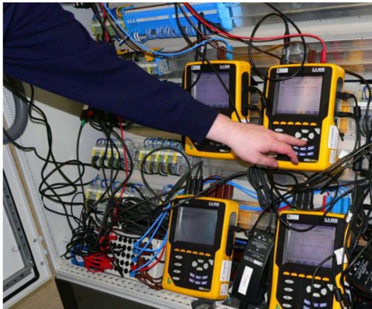
Figure 11: Typical setup of power analysers during the measurement campaign in a car manufacturing plant [5].
