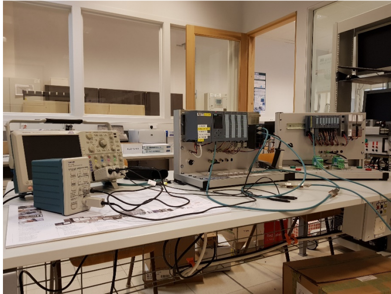
Figure 23: Overview of the set-up when measuring consumed current/power.
