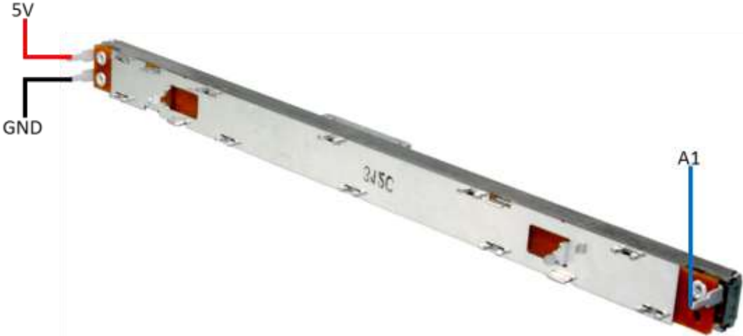
Figure 19: hardware diagram of the linear potentiometer
