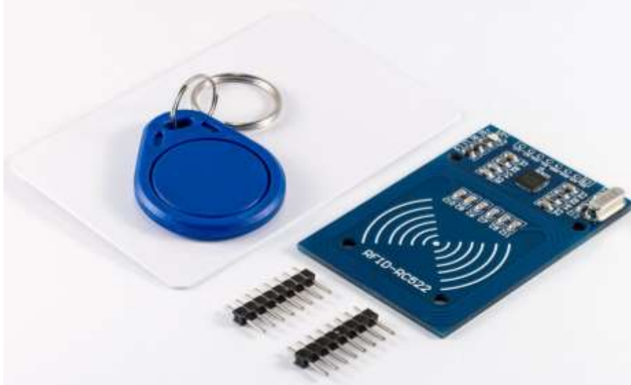
Figure 16: RFID kit image (the RC522 module, a badge and a card)
