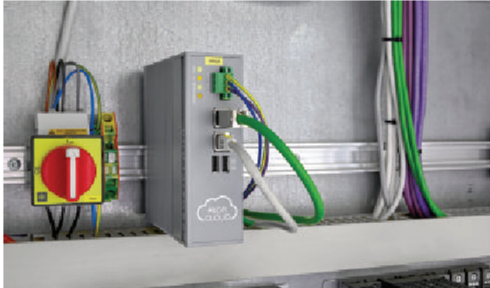
The Proficloud coupler connects the local PROFINET network to the Proficloud via two Ethernet interfaces.
