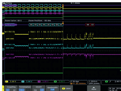
Fault generation @ 1.5 Mbps (100 m cable, B=Low, A=High) :
