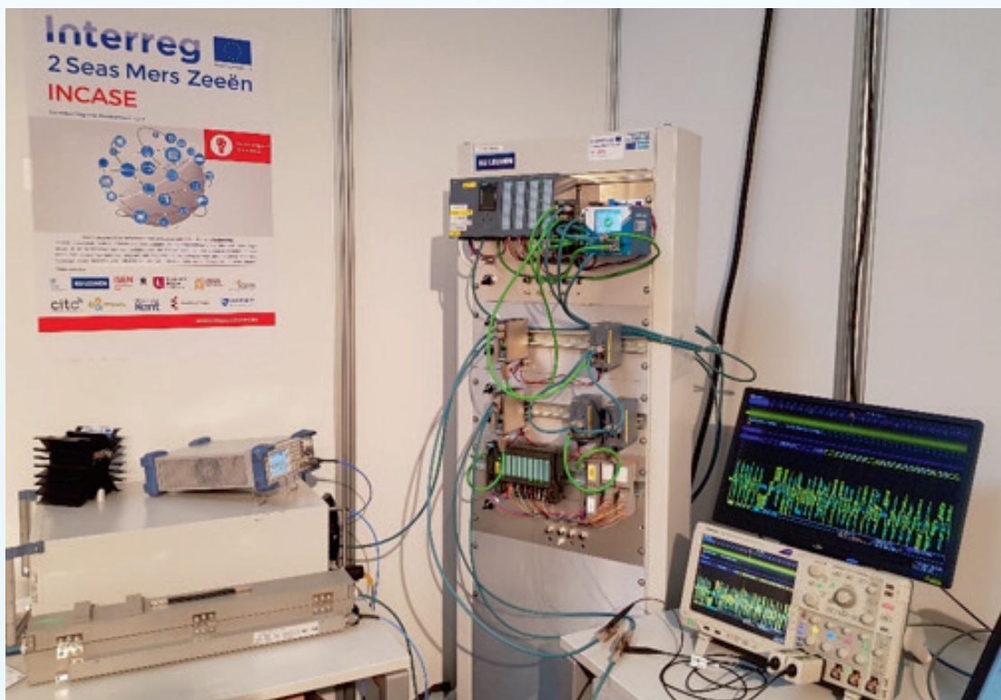
Demonstration setup at Indumation 2019: EMI coupling on a redundant PROFINET network
